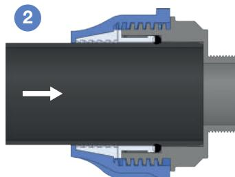
Push the pipe to the stop on the fitting.
