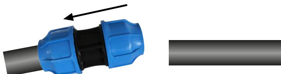
The sleeve is attached on one side of the pipe. The two pipes are aligned and the sleeve is moved to the mark on the pipe.
