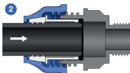
Push the pipe to the first stop (gasket) of the
