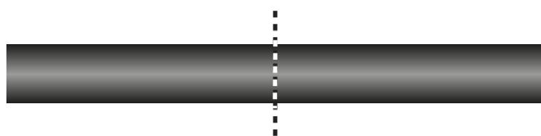
Cut the pipe perpendicular to its axis near the damaged location.
