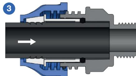
Pass the pipe through the seal and push
