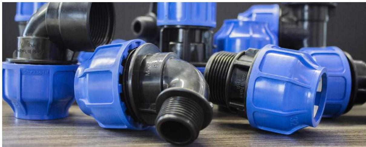
The coupling product range includes straight and reductive couplings, tees, bends, threaded connectors and end caps ranging from d20 to d110 mm and thread sizes from 1/2» to 4».
