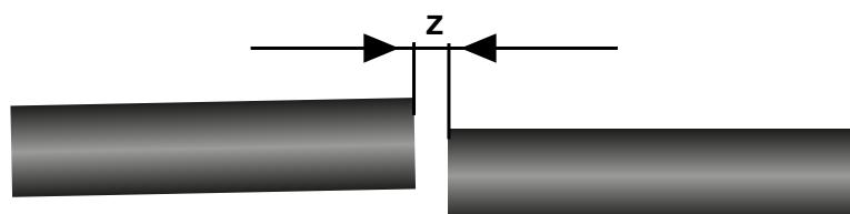
The spacing between the pipes is maintained in accordance with the pipe and fitting diameter (according to the dimensions in Table A). Pipe ends are planed approximately 15 degrees and grease is applied to the seal if necessary.
