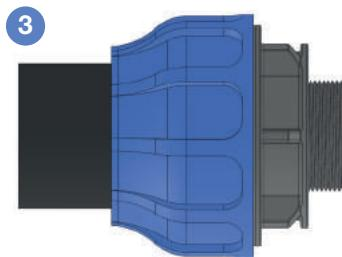
Tighten the nut to the stop ring.
