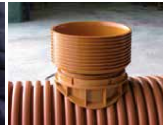
Saddle connection that corresponds to the vertical (Ø400, Ø500, Ø600) With the appropriate connector (Ø160 and Ø200) for a smooth or corrugated pipe.
